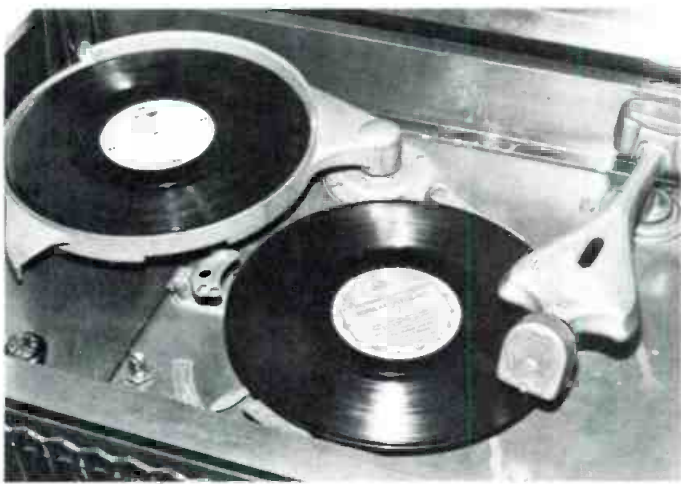
Figure 1. RCA Victor radio phonograph, 1931 model. After playing, the record was dropped onto the top of the stack and a new record was peeled from the bottom. It played 78s and Long Playing records, but only one side of 10 inch size. 12 inch records were played manually. Notice the massive size of the "Cobra Arm" pickup.
